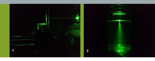
Raman laser coupled into the TopoScan system via mirror arrangement.
